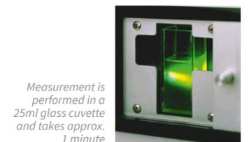
Measurement is performed in a 25ml glass cuvette and takes approx. 1 minute
