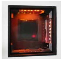
The daphnia behaviour in sample water is observed in the measuring chamber by a CCD camera
