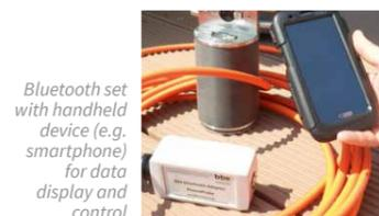
Bluetooth set with handheld device (e.g. smartphone) for data display and control
