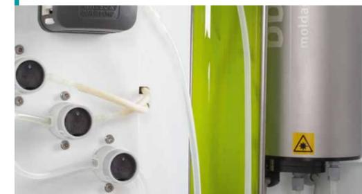
Sample water is mixed with the algae test solution and then analysed
