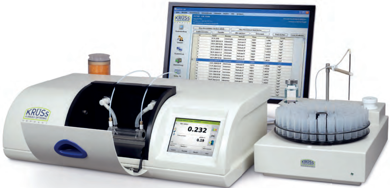
Fully automatic sample supply with P8000-TF, peristaltic pump DS7070 and autosampler AS90
